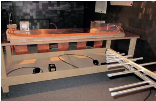
EMC test set up of a HV DC/DC converter
