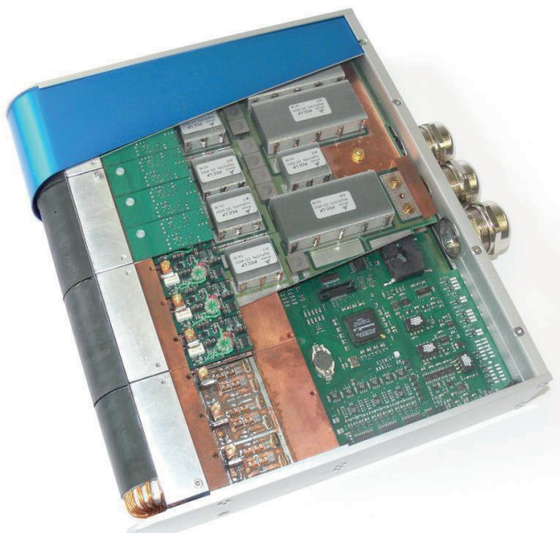
100 kW DC/DC converter with a power density of 25 kW/dm 3 and an efficiency exceeding 96% - enabled by using SiC technology
