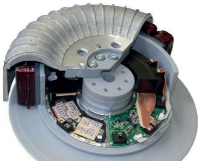
Wheel-hub-motor integrated drive inverter with 6 phases
