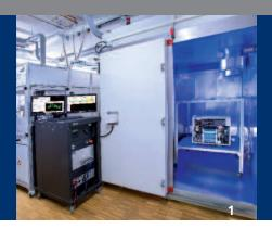
Characterization of a PEM fuel cell stack under extreme climate conditions with single cell monitoring. The system oriented stack behavior is investigated by the integration of peripheral units.
