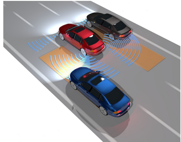
Fig. 1. The lower car (blue) is in the blind spot of the host-car’s (red) driver. The blue arcs depict the sensor range of the host-car’s us-sensors. The orange rectangles depict the critical zone which should be supervised.
