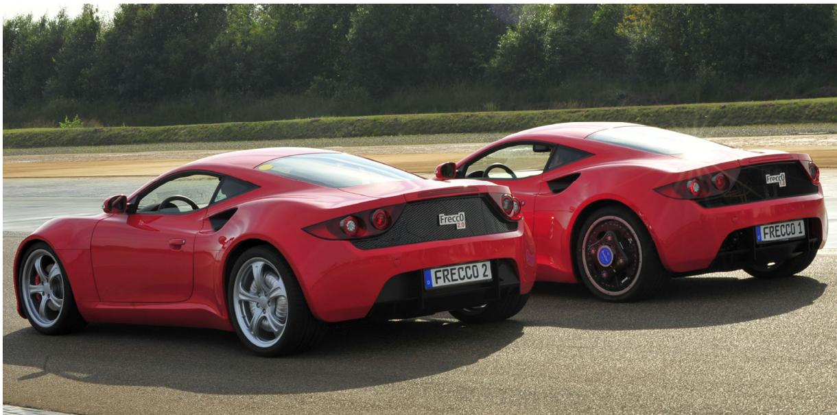
*Figure 1: Fraunhofer e-concept car Frecc0; left car: Frecc0 2.0 equipped with two electric wheel hub motors; right car: Frecc0 1.0 with electric motors near the axle (Foto: Ingo Daute / FhG)*
